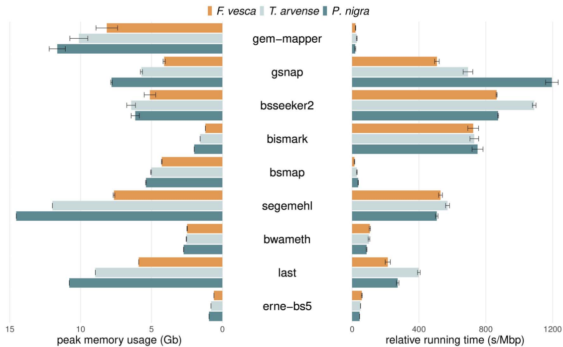
Figure 4. Peak memory and running time on alignments of simulated reads at varying levels of sequencing coverage (1–20x). Peak memory usage is given in terms of resident set size (Gb) and running time in terms of seconds per Mbp for comparison. Memory is dependant on the size of the genome relative to the effect on the index data structure, whereas time is dependant on the total quantity of reads to align. Larger error bars indicate memory usage differences that arise due to differences in sequencing depth, or non-linear increases in process running time.
