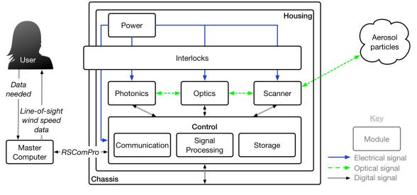
Figure 2: The OpenLidar modular wind lidar architecture [5]
