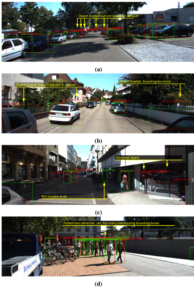
Fig. 5: Examples of error types. Green boxes refer to ground truth data, while red boxes to detections.
