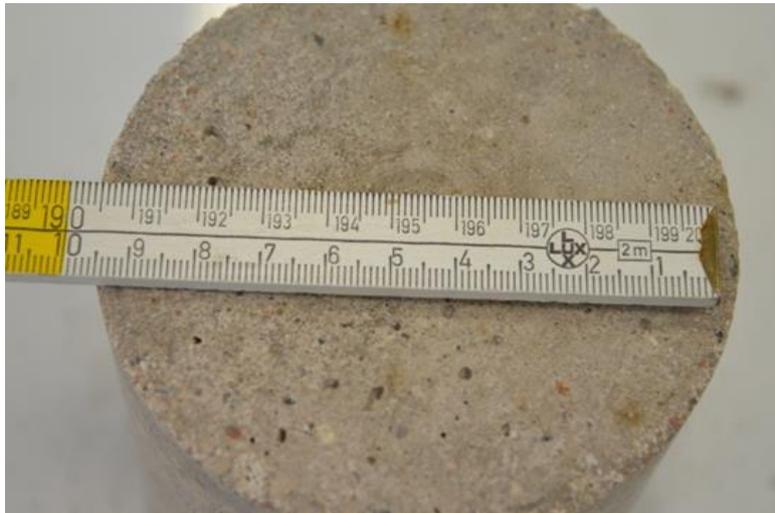
**Figure 1.** Surface of the cement stabilized sand with crushed cellular concrete and mixed recycled aggregates (0-8 mm).
