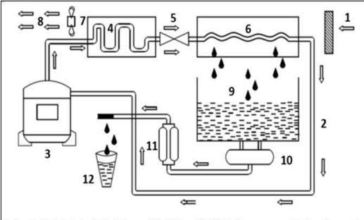
Parts: 1. Moist air In 2. Refrigerant fluid line (R-22) 3. Compressor 4. Condenser 5. Capillary tube 6. Evaporator 7. Draft Fan 8. Warm air out 9. Storage tank 10. Ozone generator 11. Water filter 12. Glass of water.
