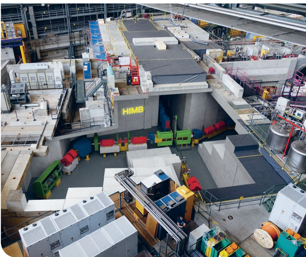
Figure 33: The planned HIMB facility utilises the Megawatt-class PSI proton beam to generate continuous low-energy muon beams with unprecedented intensity. The artist's view shows the high-intensity muon beam to the left and right of the proton-beam transmission-target station. In operation, the proton beam and target region will be covered with heavy shielding as seen further downstream (Image: PSI)
