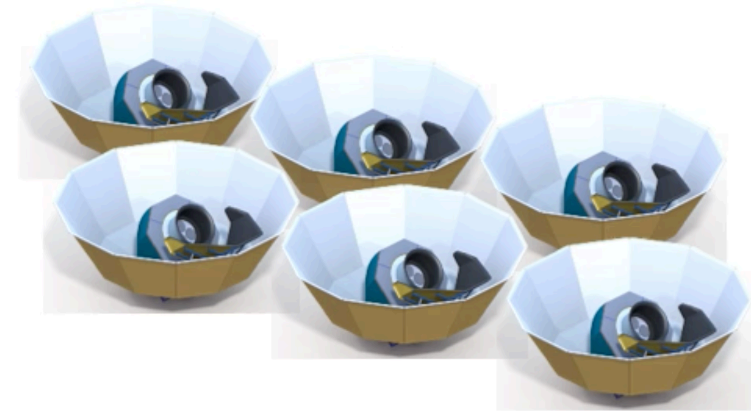
18 x 0.55m small telescopes (3 per cryostat), e.g., like BICEP Array
