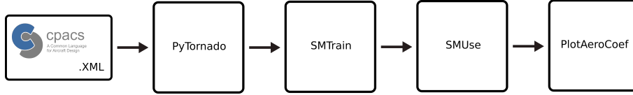
Figure 6: CEASIOMpy workflow to train and use the surrogate model for AoA prediction
