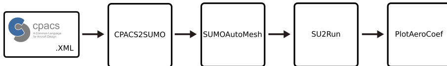
Figure 4: CEASIOMpy workflow to generate an aerodynamic database with SU2
