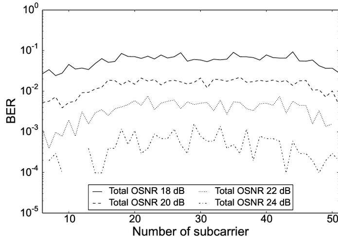
Figure 9: Distribution of BER per OFDM subcarrier.
