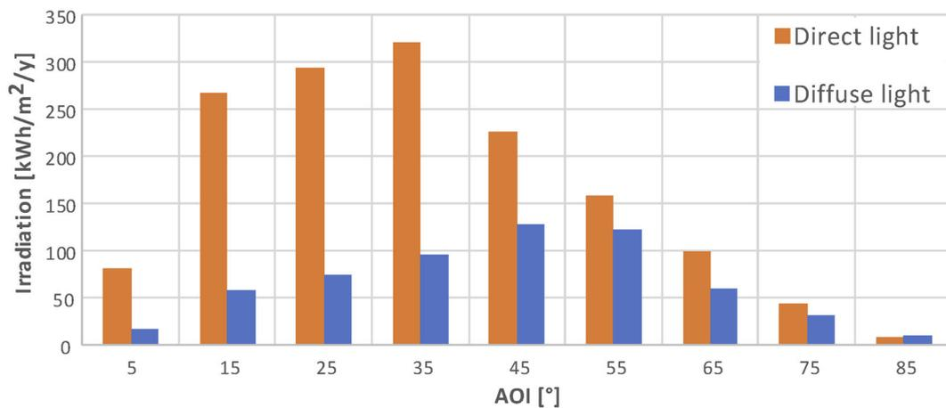
**FIGURE 7** Angular distribution ( $10^\circ$  bins) of yearly direct and diffuse inclined irradiation available in Madrid versus AOI for on a plane with a tilt of  $30^\circ$  due South
