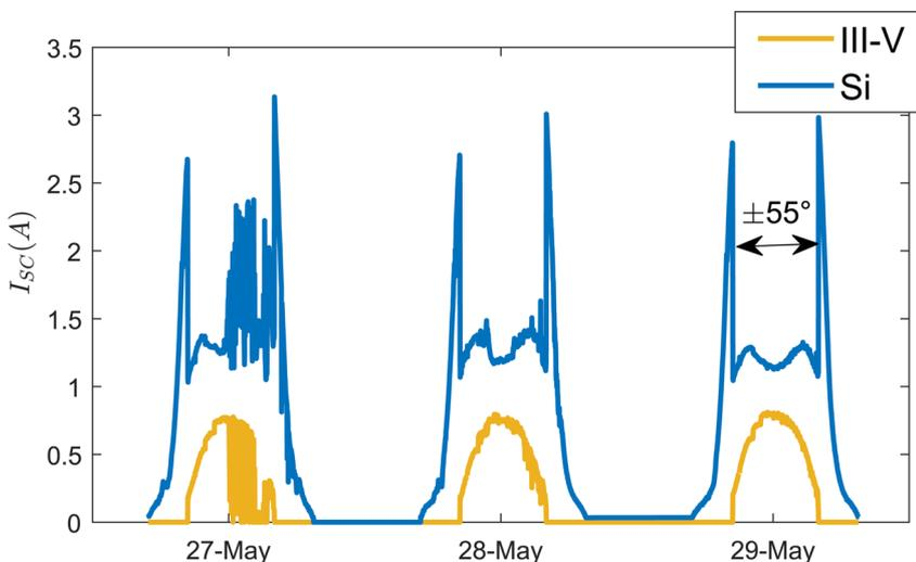
**FIGURE 2** Short-circuit current of CPV (III-V) and PV (Si) submodules monitored at the rooftop of the solar energy Institute in Madrid in 2019 during three different types of days with high DNI: afternoon cloud passages (May 27), high-altitude thin clouds (May 28), and clear sky (May 29)
