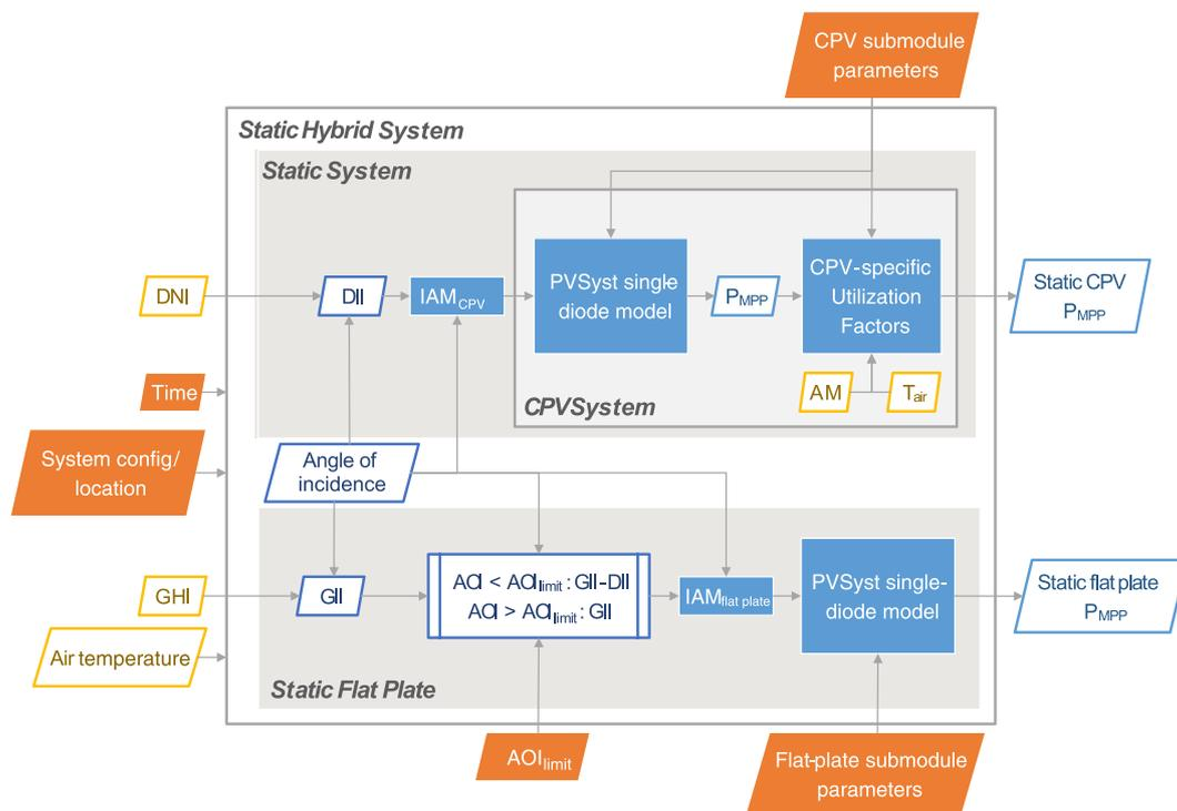
**FIGURE 11** Diagram of the PVLIB classes developed to model integrated-tracking hybrid systems composed of a CPV submodule that collects direct irradiance and a flat-plate PV submodule that collects diffuse irradiance
