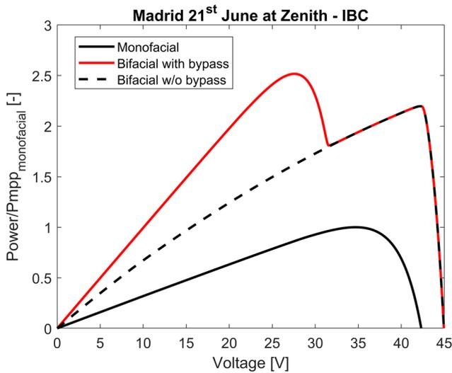
**FIGURE 15** Power plot normalized by the  $P_{mpp}$  in monofacial configuration. Simulation uses synthetic clear sky conditions (Ineichen model) on June 21 at zenith time and for a 300-cm ground clearance
