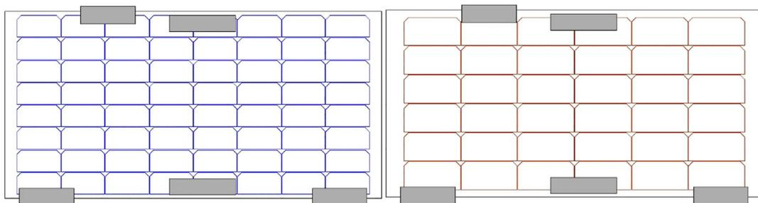
**FIGURE 13** Left: configuration A with eight strings of eight half-cut IBC solar cells. Cells are connected in series along the long dimension. Right: configuration B with six strings of six half-cut HJT solar cells. Cells are connected in series along the small dimension. The gray rectangles are module components inducing shading on the rear side of the Si cells. Each string is connected in parallel with a bypass diode
