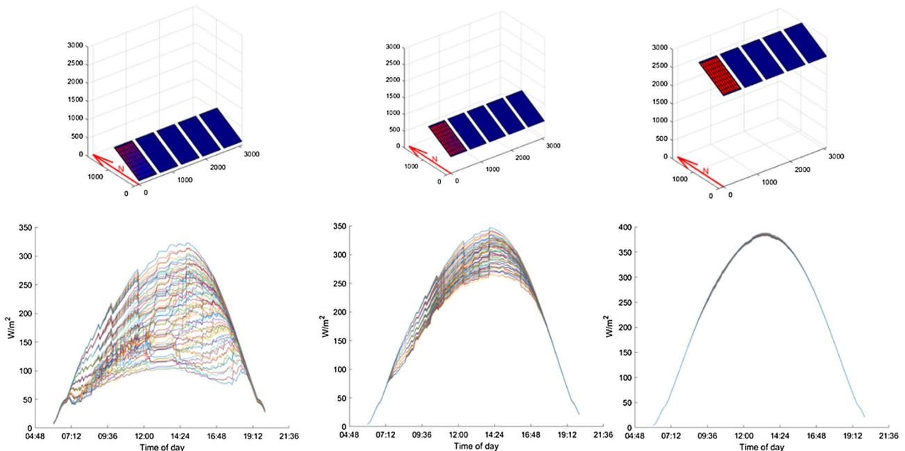
**FIGURE 14** Top: colmap of the simulated irradiance reaching each cell on the rear side for three different ground clearance—0, 50, and 300 cm. Bottom: rear irradiance reaching the cells during a day under clear sky conditions (Ineichen model). Each line represents a unique cell
