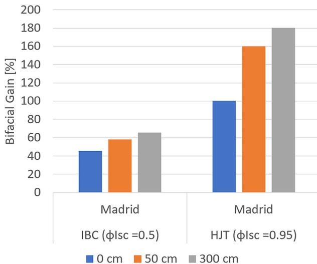
**FIGURE 16** Estimated bifacial gains on the yearly energy yield for configurations A and B in Madrid at three different ground clearance heights. Please note that the front side receives diffuse irradiance only. For comparison, 40% bifacial gain is obtained in the 50-cm-clearance simulation setup for bare flat-plate HJT modules (without the CPV cover)
