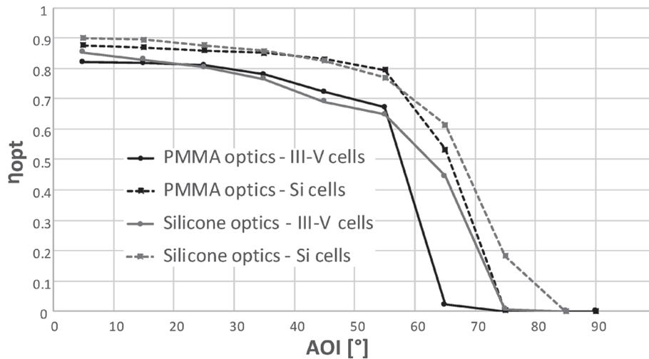
**FIGURE 5** Angular performance of the lens design: optical efficiency as a function of AOI for concentration onto a III–V cell (continuous lines) and for light transmission to a Si cell (dashed lines). Two optical designs are shown: silicone lens design (gray lines) and PMMA lens design (black lines)
