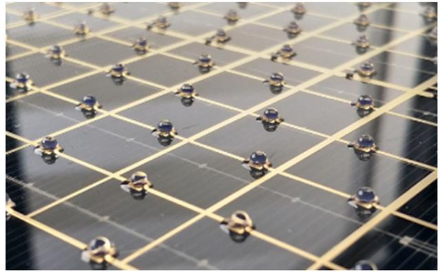
**FIGURE 3** Photograph of the backplane of the glass-Si-glass laminate for the Insolight III-V/Si hybrid architecture: III-V cells are assembled on a transparent printed circuit board, which is laminated on top of Si cells (multi-busbar PERC cells in this case, although several alternatives have been studied). III-V cells are encapsulated under secondary optics (half-ball lenses) to increase alignment tolerances
