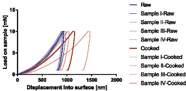
Fig. 3. Average Load vs. Displacement curves for raw and cooked bone
