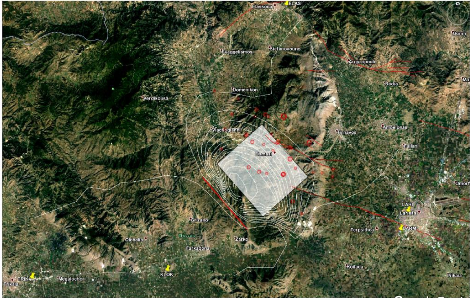
Figure 1. Location of the picked fringes, projection of the model 3 fault, location of some GNSS points. Location (EMSC) of the first aftershocks. Faults from the NOA v3.0 data base.
