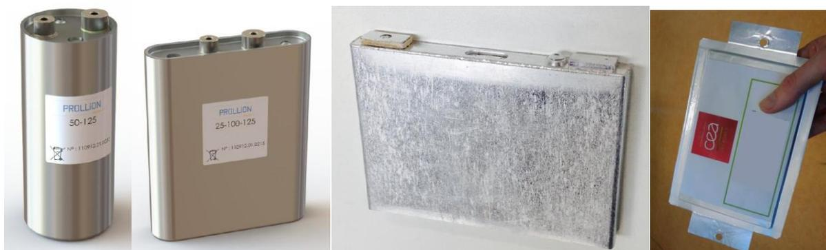
**Figure 1.** Picture of the four types of cell packaging that will be produced within SPICY. From Left to right: Cylindrical hard casing 17 Ah (PROLLION), Prismatic hard casing 17 Ah (CEA), Prismatic hard casing 5 Ah (TUM), and prismatic soft packaging (pouch Bag) 17 Ah (CEA).
