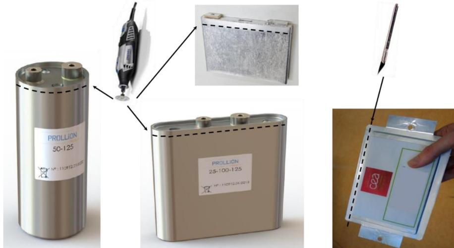
**Figure 2.** Sketch of opening cuts (precise cuts to be defined in [January - March] 2016)
