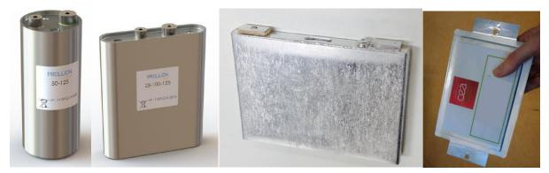
**Figure 1.** Picture of the four types of cell packaging that will be produced within SPICY. From Left to right: Cylindrical hard casing 17 Ah (PROLLION), Prismatic hard casing 17 Ah (CEA), Prismatic hard casing 5 Ah (TUM), and prismatic soft packaging (pouch Bag) 17 Ah (CEA).
