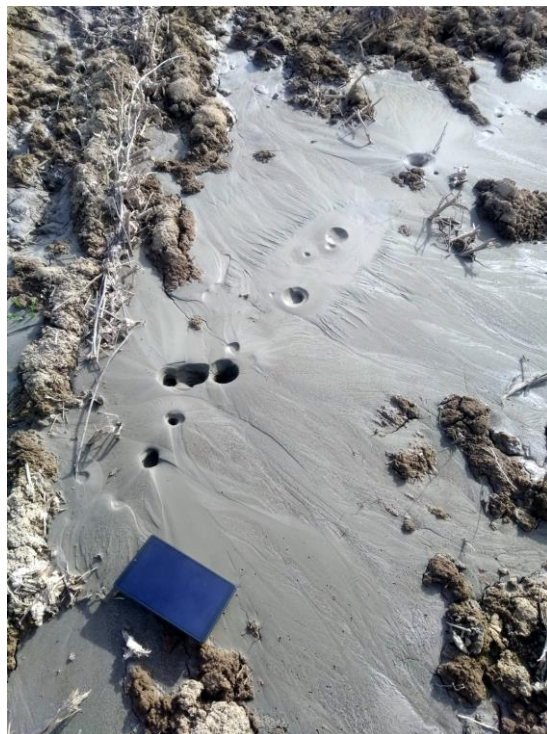
Figure 15. Close-up of liquefaction fissure with small craters (Photo taken by S. Valkaniotis 05/03/2021).
