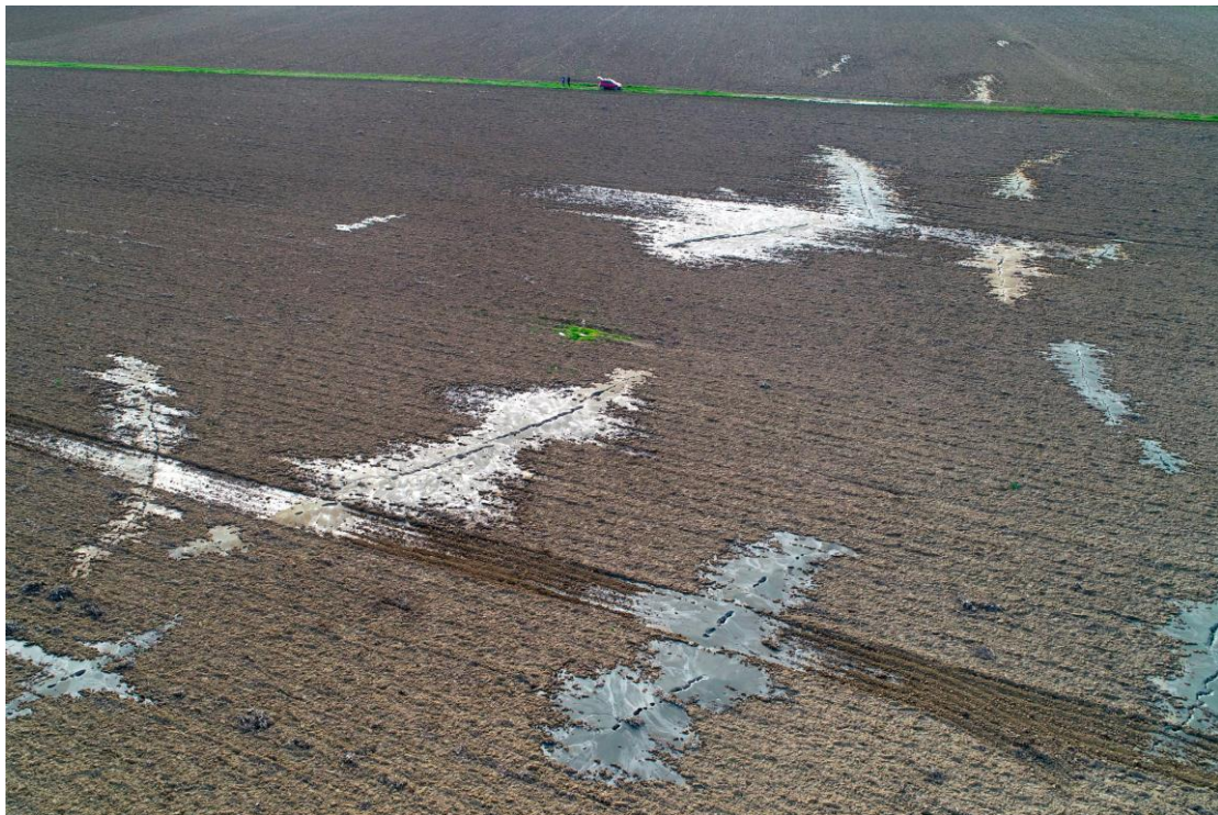
Figure 11. Aerial view of multiple linear liquefaction fissures (Photo taken by G. Papathanassiou 05/03/2021).
