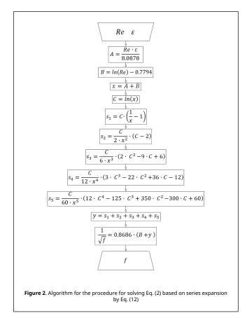
Besides, if  $y \approx s_1$ , Eq. (8), the relative error is up to 0.153% with around 0.2 seconds for the execution of 8 million of Quasi Monte-Carlo tested samples. Based on the algorithm from Figure 2 and using only  $y \approx s_1$ , Eq. (21) can be constructed (this equation is already presented in [21])
