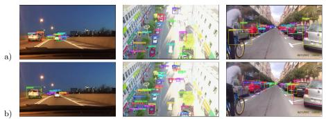
Fig. 4: Object detection results obtained from the application of the Mask R-CNN (a) and Flow R-CNN (b) models to the supported datasets[29, 30, 4]
