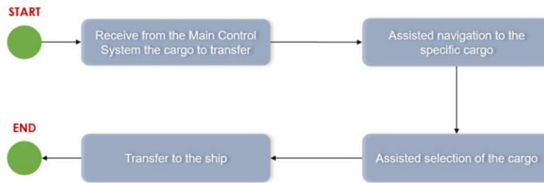
Figure 4 Procedure Diagram — Transfer to Crane
