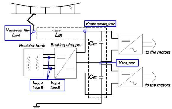
Fig. 1. Scheme of the E464 traction architecture, identification and positioning of the monitored quantities
