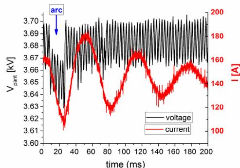
Fig. 9. Effects of arc voltage events measured at the voltage and current at the pantograph
