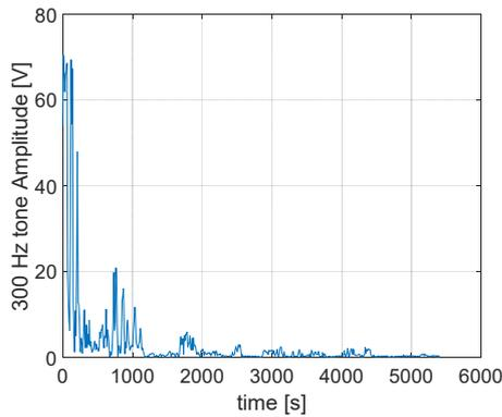
Fig. 11. Behavior of the 300 Hz pantograph voltage ripple along the Bardonecchia – Torino line
