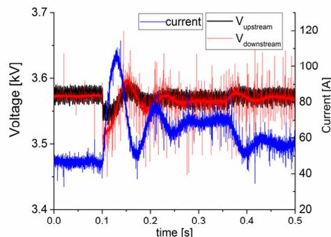
Fig. 10. Effects of the insertion of an auxiliary burden on the current and voltage at the pantograph and voltage downstream the filter
