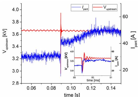
Fig. 8. Voltage and current at the pantograph during a fast transient event.
