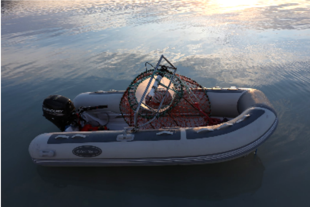
The RBR CTD was mounted to a lobster trap and deployed overnight near the terminus of Eqip Sermia. The pressure sensor recorded waves that were generated by calving events.
