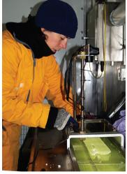
Figure 1.28 A sea ice scientist is using polarising filters to examine an ice sample.
