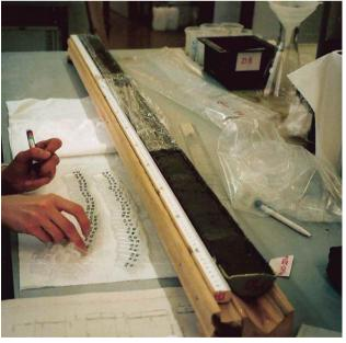
Figure 1.48 A lake sediment core is being subsampled for diatom analysis.
