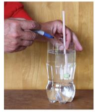
Figure 1.23 Calibrating the hydrometer.
