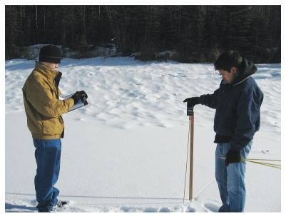
Figure 3.2 Measuring the snow depth and the snow-ice interface temperature with a temperature probe and digital reader.
