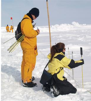
Figure 3.23 Teacher Caroline Lapworth and a researcher measuring temperature at the snow/ice interface.
