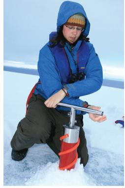
Figure 3.12 Student taking an ice core sample.
