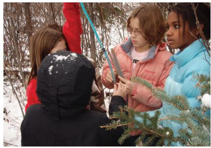
Figure 3.4 Students measuring depth of soil freezing using the frost tube protocol.
