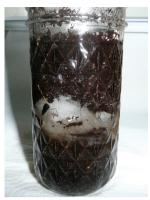
Figure 1.57 Prepared 'permafrost' sample.
