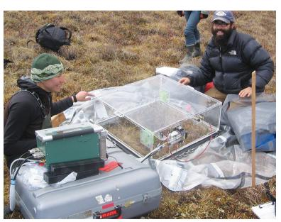
Figure 3.30 Measuring CO<sub>2</sub>-flux,Toolik Field Station, northern Alaska.
