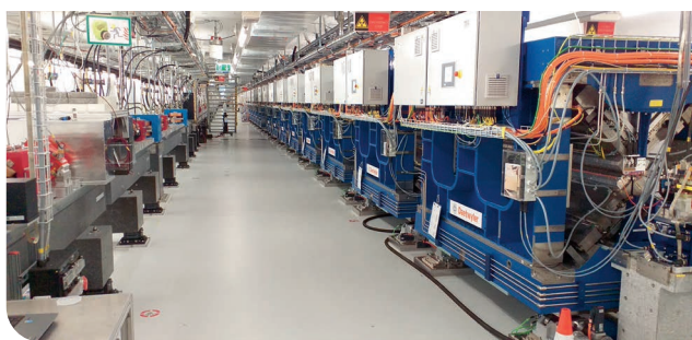
Figure 16: A part of the undulator array for Athos.
