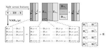
Fig. 1. Definition of  $VAR_n(p)$  model and data structure.
