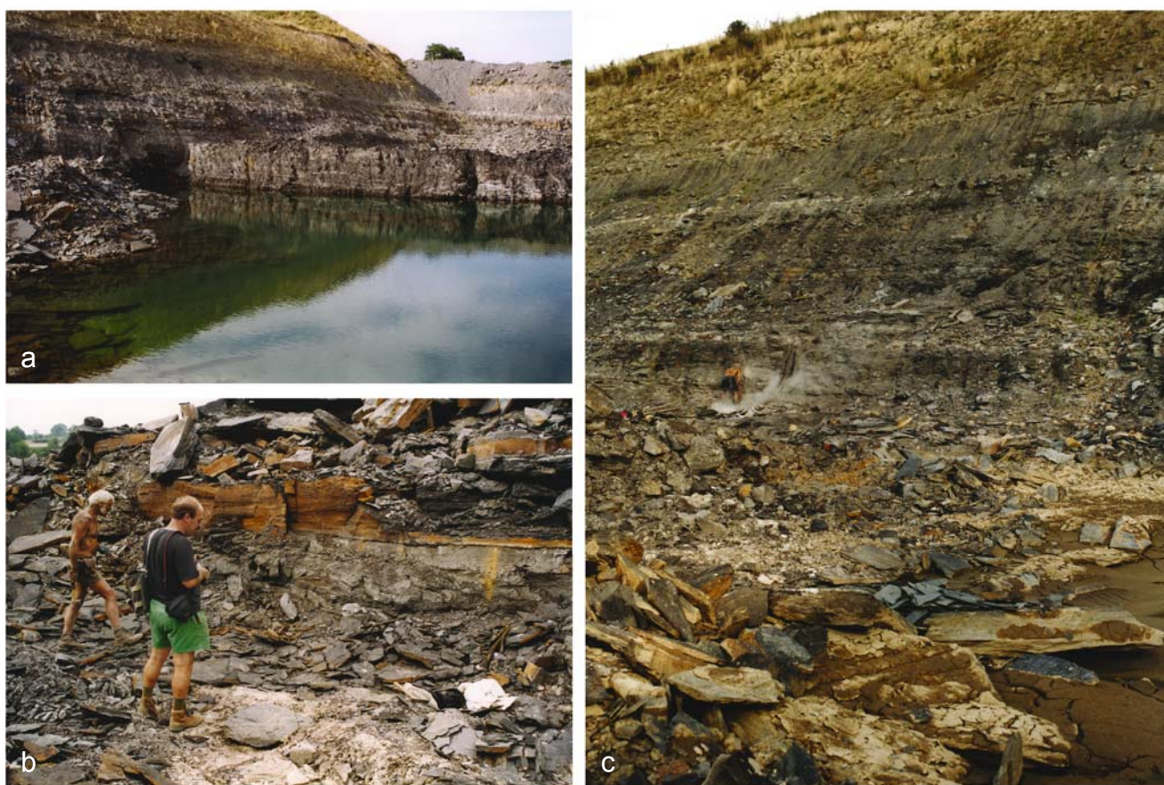
Text-fig. 2. Opencast coal mine in Buxières-les-Mines in the year 1999. a – flooded area after mining of coal seam. b – section of lacustrine bituminous black shales with fauna. c – 30 m thick section of lacustrine bituminous black shales, fluvial clastics and channel sandstones in the mine.
