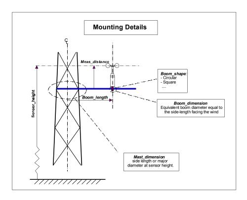
Figure C-1: definition of mounting details.
