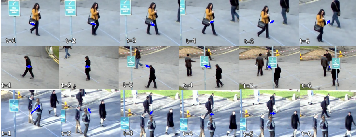
Figure 8: Samples of Sequences: (a) Seq1: Following 1 and then 2 targets. Notice that the network decides to move towards the center of mass of the two targets. (b) Seq2: The network follows a single target then it moves to the center of the group. Also the network does not move away from the partially occluded target. (c) Seq3: Multiple targets present the network adjusts to the movement of incoming targets.
