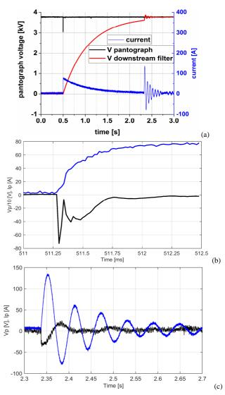
Fig. 3. Measured waveforms of pantograph voltage  $V_p$ , pantograph current  $I_p$  and capacitor voltage downstream of filter  $V_j$ : (a) overall screenshot of the relevant time interval, (b) zoom of the first insertion with resistor  $R_{ch}$ , (c) zoom of the residual oscillation when the resistor  $R_{ch}$  is bypassed.
