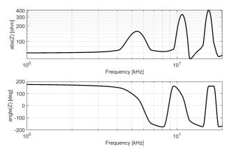
Fig. 6. Identified network impedance  $Z_n$  after calculation of cross- and auto-spectrum, ratio, compensation of the electric parallel with the onboard filter, and interpolation to visually improve frequency resolution.
