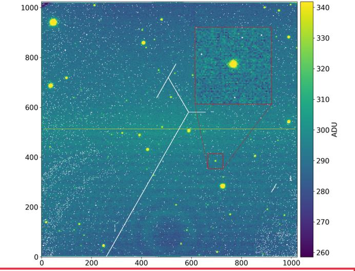
A reduced PINES field taken in *J*-band with Mimir, with bad pixels represented in white. The region surrounding the target L dwarf is shown in the inset. Mimir data has a number of cosmetic issues, including a crack in the detector running from the lower left to the middle of the image. Bad pixel values are corrected if they fall within a target or reference aperture in the PINES Analysis Toolkit.
