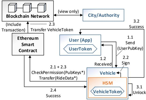
Fig. 4. Unlocking and permission validation procedure
