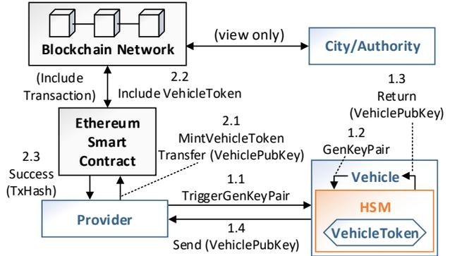
Fig. 3. Vehicle registration procedure triggered by provider
