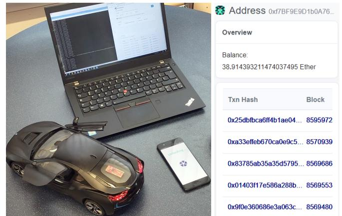
Fig. 5. Proof-of-concept with implemented HSM and test transactions performed in *Ropsten Testnet* (<https://ropsten.etherscan.io/>)
