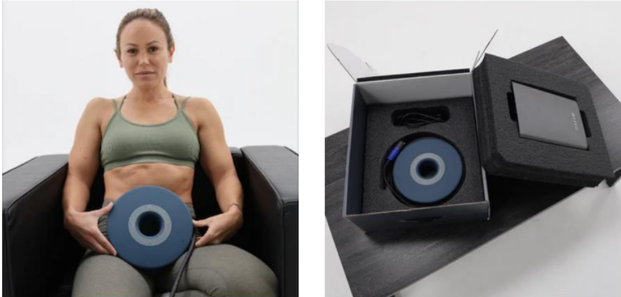
Figure 2. The HAELO device consists of a Symphony One unit and coil with recommended placement on the abdomen, chest, or specific areas of muscle soreness or injury.
