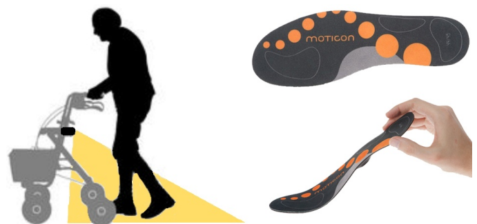
Figure 2: Instrumentation of our wheeled walker (left), utilized wireless insole “Moticon OpenGo” sensor (right)
