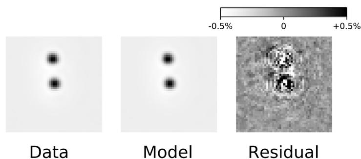
Relative astrometry is obtained by subtracting a model system from the observed data, utilising a grid-search approach in  $x$ - and  $y$ - positions as well as brightness scaling for the components until a minimum residual is obtained. The figure depicts the typical quality of the two major contributing sources of data for the survey, with a precision on the order of a few milliarcseconds.
