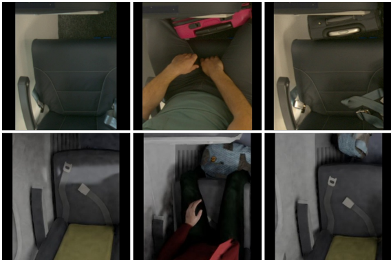
Figure 9: Real (top) and synthetic (bottom) ROI samples for training a classification DNN with correct and incorrect situations.
