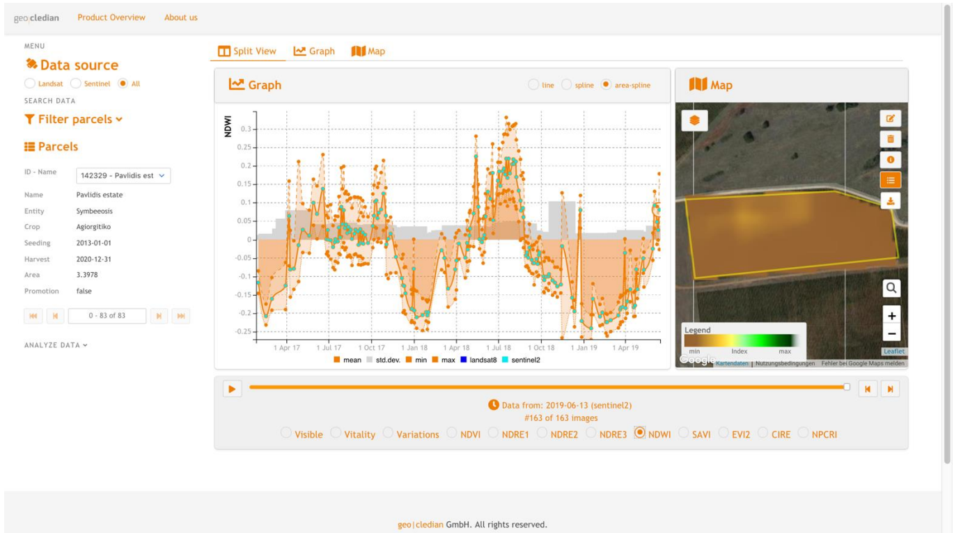
Figure 5: A Sentinel-2 NDWI time series for 2017 - 2019 for a parcel of the Pavlidis estate, Greece showing also the NDVI image for 13th June 2019. This NDWI is known to be related to leaf water content.
