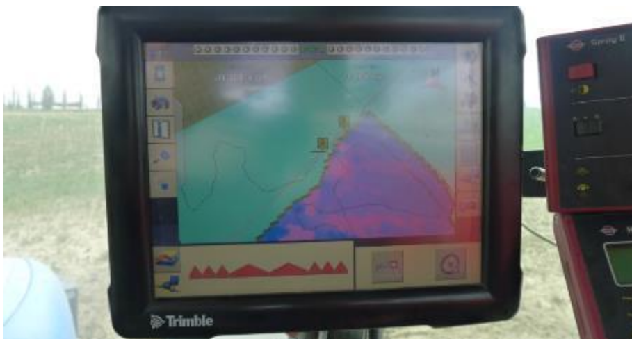
Figure 21 Import of a prescription map on a Trimble VR computer
