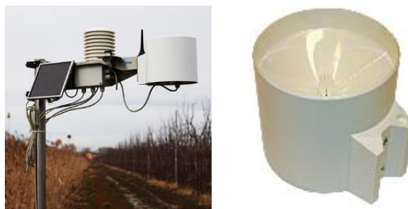
Figure 5 Sensor & Weather Station (left) and Rain Gauge Module (right)
