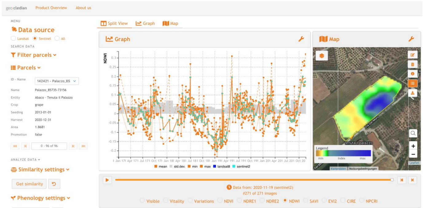
Figure 10 A Sentinel-2 NDWI time series for 2017 – 2020 for a parcel of the Tenuta il Palazzo vineyard, Italy. This NDWI is known to be related to leaf water content.
