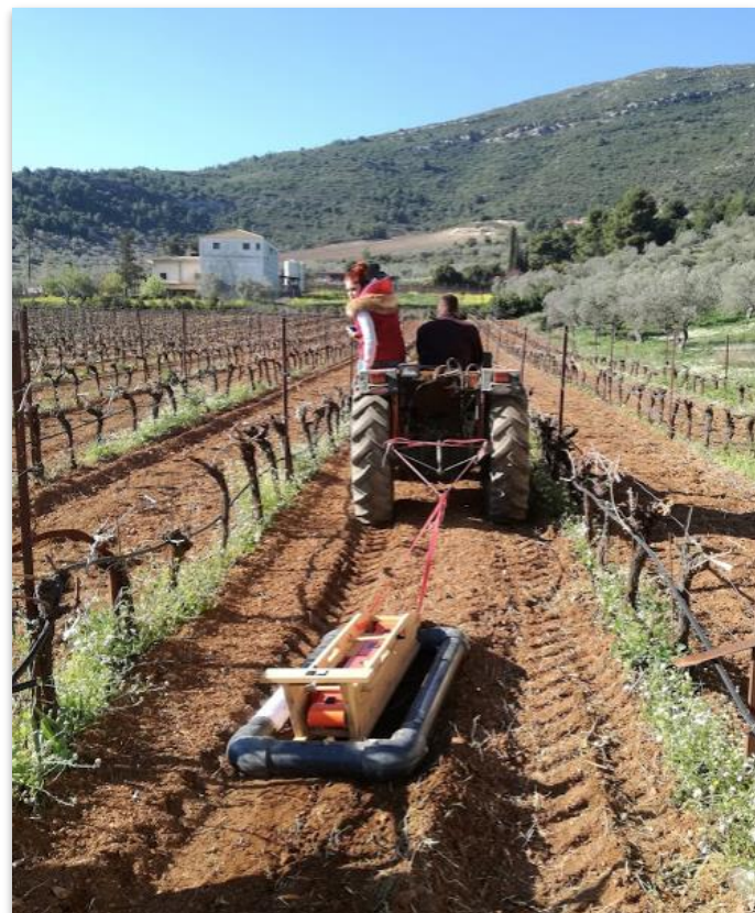
Figure 5: EM38-MK2 placed on its sleigh
