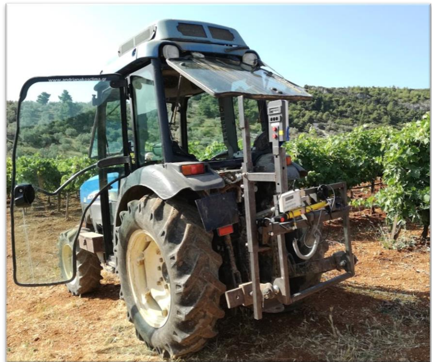
Figure 9: Both canopy sensors mounted on a tractor
