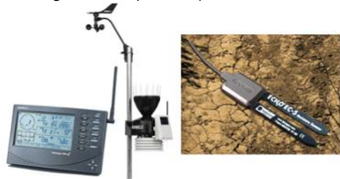
Figure 11: Vantage Pro2 Weather Station (left) and Decagon EC-5 soil moisture sensor (right)
