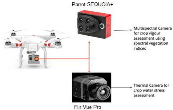
Figure 10: Phantom 4 Pro drone equipped with multispectral or thermal camera
