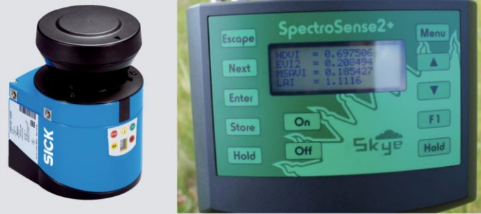
Figure 7. Laser Scanner LMS100 (left) and SpectroSense2+ (right)
