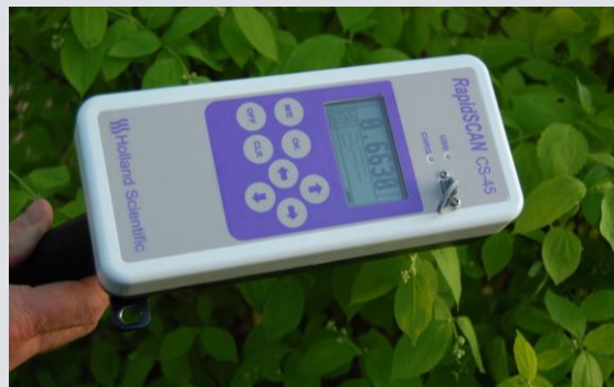
Figure 8: Crop Circle RapidSCAN AC-45 handheld reflectance sensor
