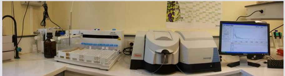
Figure 16: SAFAS UV-mc2 Spectrophotometer
