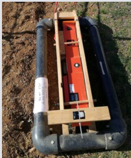
Figure 4: EM38-MK2 (left) and Archer Data logger (right)
