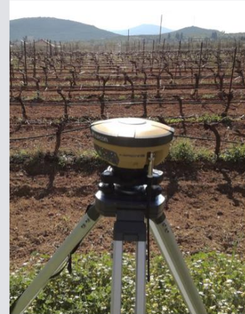
Figure 5: Topcon HiPer V RTK GPS
