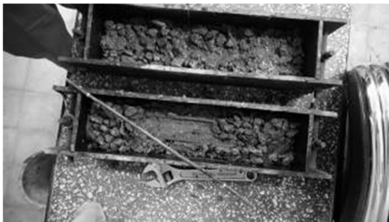
Fig. 2. Casting TC into the mold.
