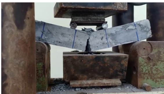
Fig. 8. Failure mode at the middle third due to bending.
