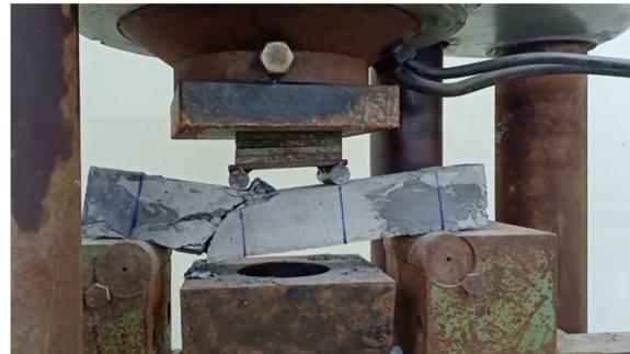
Fig. 9. Failure mode at the left third due to shear.
