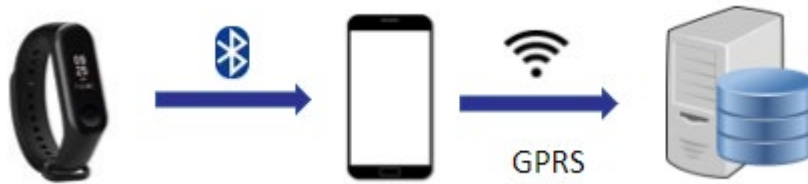
Figure 6.8.1 Sensor data generation and communication
