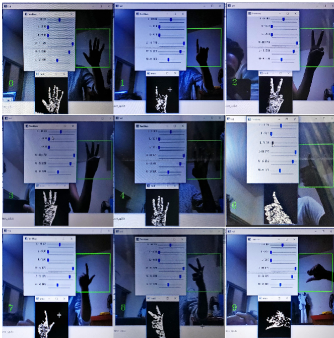
Fig. 24. Real time recognition of Bengali Sign Language (Digit) using CNN
