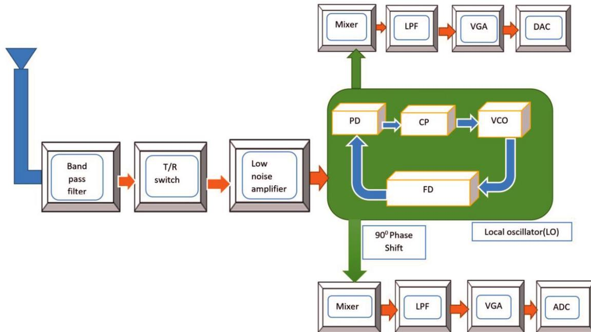
Figure 1. A typical RF receiver front-end
