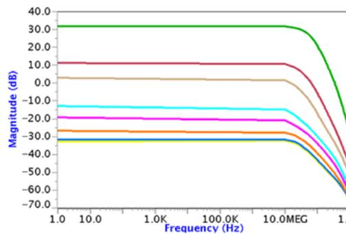
Figure 4. Gain responses by varying feedback resistor ( $R_f$ )
