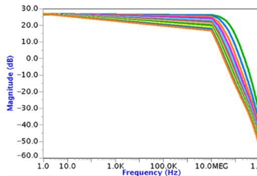
Figure 5. Gain responses by varying source degeneration resistor ( $R_s$ )
