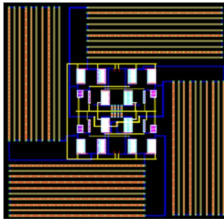
Figure 7. Core layout of the proposed VGA circuit
