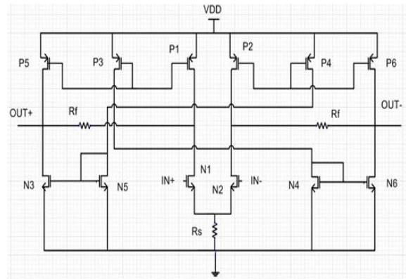
Figure 3. Schematic of the single stage of the VGA circuit
