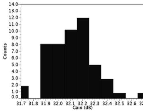
Figure 6. Monte Carlo analysis of the VGA for maximum gain
