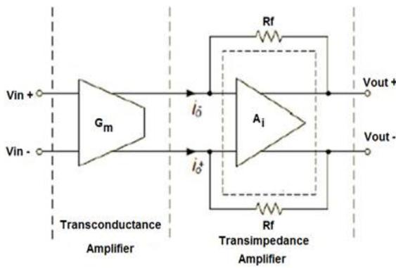
Figure 2. Design of the single stage variable gain amplifier circuit
