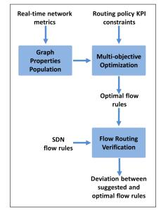
Figure 2. The workflow of the proposed flow routing policy verification methodology: based on the topology of the network (formulated as an undirected graph), and the routing policies, multi-objective optimization is applied in order to compute the optimal flow rules. These optimal rules are then compared with the flow rules of the SDN in order to identify discrepancies.
