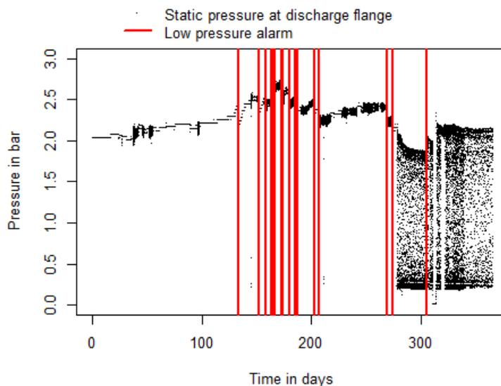
Figure 4: Evolution of the static pressure at the discharge flange.
