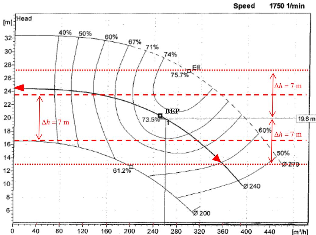
Figure 5: Characteristic of the sea water cooling pump, showing the potential deviations from the BEP.
