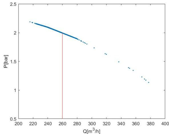
Figure 7: Observed variation of the measured discharge pressure and the pump flow (estimated from pressure).
