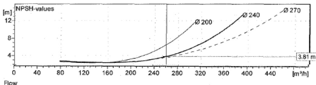
Figure 6: Net positive suction head at different flow values.
