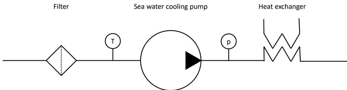
Figure 2: Simplified layout of the sea water cooling system, including sensors measuring the pressure (p) and temperature (T).
