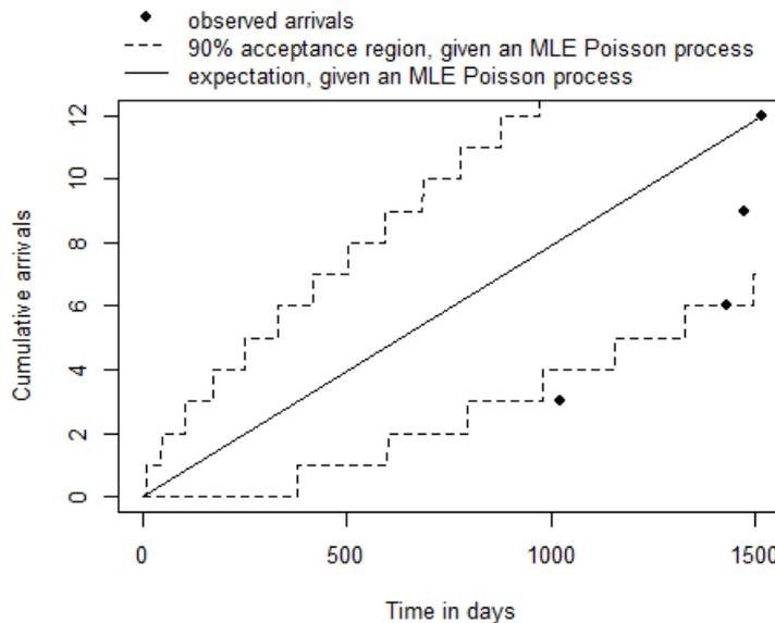
Figure 3: Arrivals of impeller failures in time (solid points) and expected failures (line + confidence bounds) when assuming a homogeneous Poisson process.
