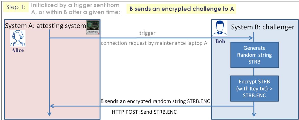
**Fig. 3-4. Trusted Hardware based principle of challenge and response: Step 1 – the challenge –**
