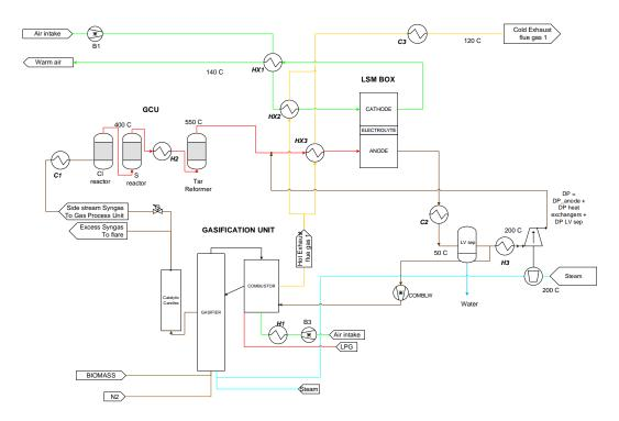
Figure 13. Option B process flow diagram of the BLAZE pilot plant. The AOG is sent to the SOFC LSM inlet stream (RR = 0.5) and the rest is burnt in the gasifier combustor. The recirculator condenses water before recycling (provided by HyGear, modified by EPFL LAMD and GEM). C: cooler; H: heater.
