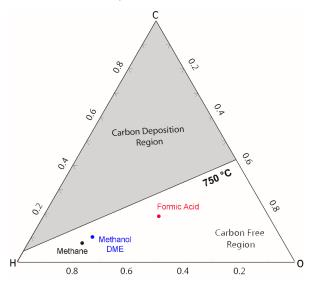
Figure 1. Equilibrium carbon deposition boundaries for the CHO system for 750 °C and O/C = 2, for different carbonaceous fuels (source: EU BALANCE project, D5.1).
