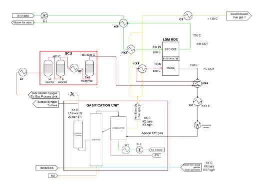
Figure 14. Option D process flow diagram of the BLAZE pilot plant. The AOG is sent to the gasifier combustor. The recirculator is not used (provided by HyGear, modified by EPFL LAMD and GEM). C: cooler; H: heater.
