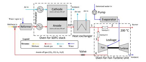
Figure 5. Recirculator integrated for a 6  $\rm kW_e$  stack with natural gas as feedstock (provided by EPFL LAMD).
