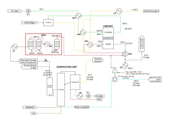
Figure 11. Option C process flow diagram of the BLAZE pilot plant, with a pressurised gasifier. Option G is analogous; instead of using a pressurised gasifier, it counts with a suction blower B2, after C1. The AOG is sent to the SOFC LSM inlet stream (RR = 0.5) and the rest is burnt in a downstream burner (provided by HyGear, modified by EPFL LAMD). C: cooler; H: heater.
