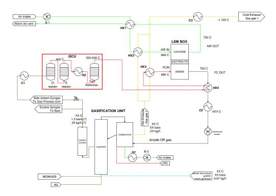
Figure 12. Option D process flow diagram of the BLAZE pilot plant, with a pressurised gasifier. The AOG is exclusively burnt into the gasifier combustor. The recirculator is not used (provided by HyGear, modified by EPFL LAMD). C: cooler; H: heater.
