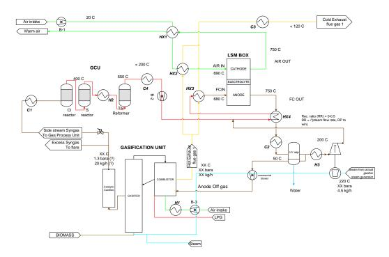
Figure 15. Option F process flow diagram of the BLAZE pilot plant. The AOG is sent to the SOFC LSM inlet stream (RR = 0.5) and the rest is burnt in the gasifier combustor. The recirculator condenses water before recycling. The gasifier is not compressed and the suction blower is placed after the GCU, after the cooler C4 (provided by HyGear, modified by EPFL LAMD and GEM). C: cooler; H: heater.
