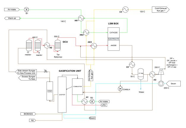
Figure 16. Option B process flow diagram of the BLAZE pilot plant. The AOG is sent to the SOFC LSM inlet stream (RR = 0.5) and the rest is burnt in the gasifier combustor, with heat exchange (same configuration for options D – Figure 14 and F – Figure 15; PFD F has moreover a cooler, C4, downstream the tar reformer) (provided by HyGear, modified by EPFL LAMD and GEM). C: cooler; H: heater.
