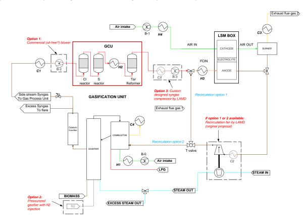
Figure 8. Process flow diagram of the BLAZE pilot plant, showing the recirculation options 1 and 2 and the possible custom designed compressor (option 3) (provided by HyGear, modified by EPFL LAMD). C: cooler; H: heater.
