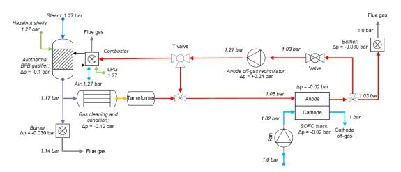
Figure 6. Example of calculation of the pressure drop / rise along the relevant BLAZE plant streams, considering a pressurised gasifier (provided by EPFL LAMD).
