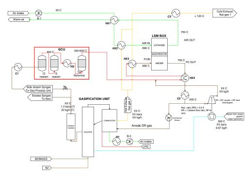
Figure 10. Option B process flow diagram of the BLAZE pilot plant, with a pressurised gasifier. Option F is analogous; instead of using a pressurised gasifier, it counts with a suction blower B2, after C1. The AOG is sent to the gasifier combustor and to the SOFC LSM inlet stream (RR = 0.5) (provided by HyGear, modified by EPFL LAMD). C: cooler; H: heater.
