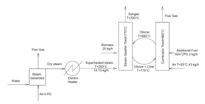
Figure 3. Detail of the DFBFG (provided by UNIVAQ).
