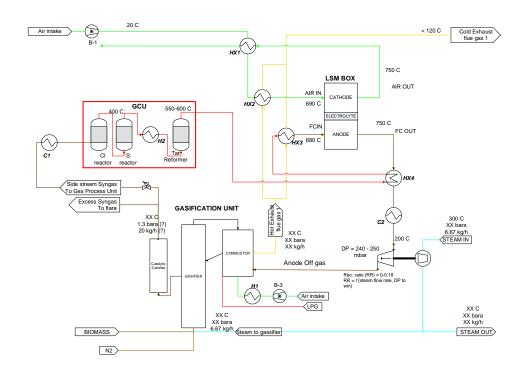
Figure 9. Option A process flow diagram of the BLAZE pilot plant, with a pressurised gasifier. Option E is analogous; instead of using a pressurised gasifier, it counts with a suction blower B2, after C1. All the AOG is sent to the gasifier combustor (provided by HyGear, modified by EPFL LAMD). C: cooler; H: heater.
