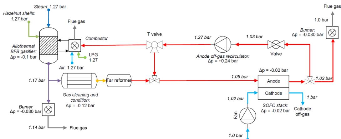
Figure 6. Example of calculation of the pressure drop / rise along the relevant BLAZE plant streams, considering a pressurised gasifier (provided by EPFL LAMD).
