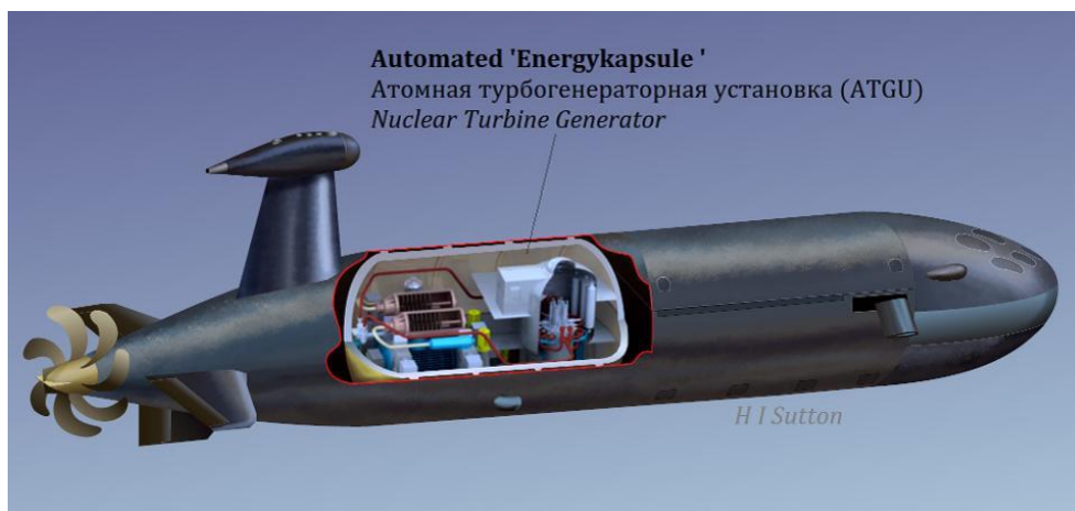
Figure 5: Conceptual illustration of un-crewed nuclear powered attack submarine built around the Russian Automated Nuclear Turbine Generator
