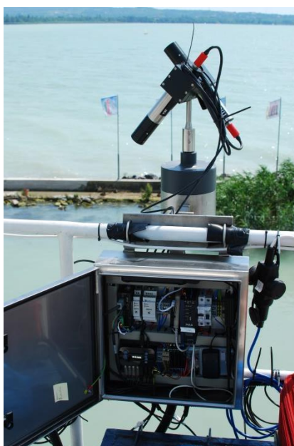
Figure 2 The So-Rad system mounted on a car ferry on Lake Balaton in June – July 2019, showing the two radiance sensors on a rotating enclosure (top) and the integrated controller and power supply box (bottom).
