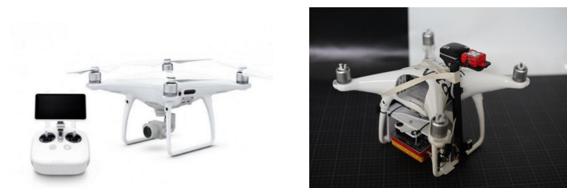
Figure 8 Prosumer drone system: (l) the default DJI Phantom 4 pro, (r) DJI Phantom 4 pro with multispectral camera MicaSense RedEdge-M mounted underneath.
