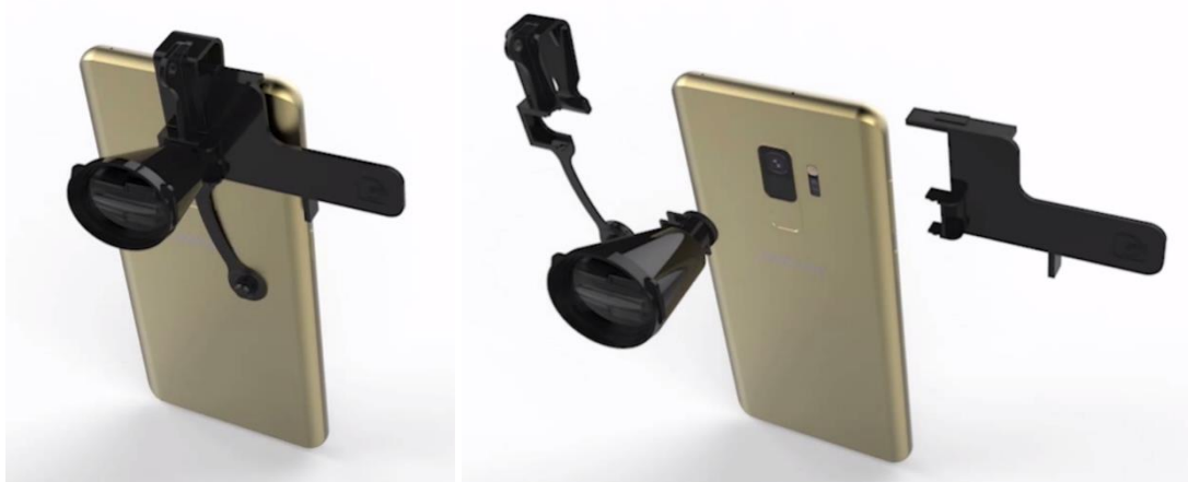
Figure 48 3D model of the iSPEX 2 add-on mounted on a smartphone. Left: full add-on. Right: exploded view.
