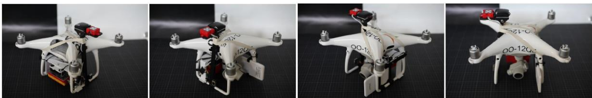
Figure 9 Final result of the integration of the MicaSense RedEdge-M camera under DJI Phantom 4 pro drone platform
