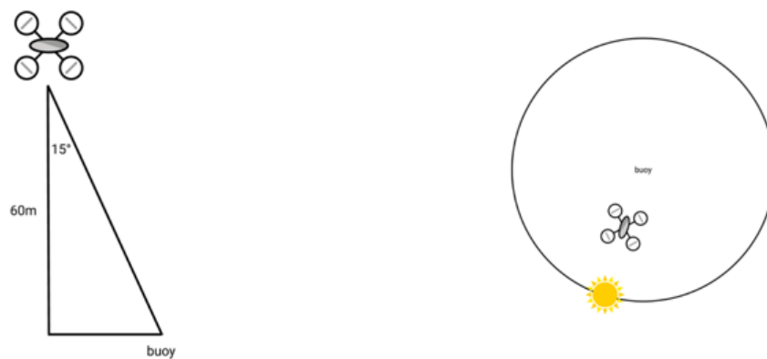
Figure 11 Schematic view of the coordinate shifter: with a tilted camera, the coordinates of the drone are slightly shifted compared to the coordinates of the buoy (left). The direction depends on the location of the sun (right).
