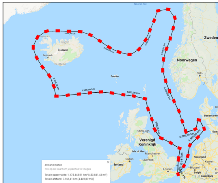
Figure 13: Example of a fully submerged mission with a hybrid-electric submarine design (maximum range of 3850 nm is attained at a speed of 5.2 knots). Snorting moments of the reference design are indicated in red. Figure adopted from (Venema, 2019).
