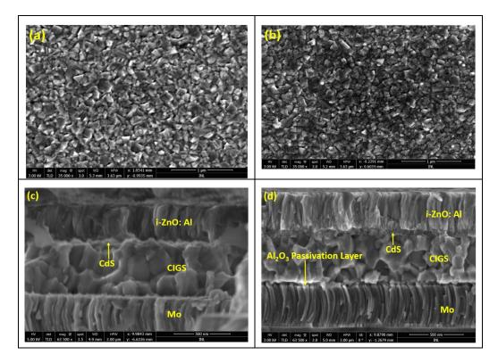
Fig. 3. Scanning electron microscopy images taken in different magnifications. (a) shows the CIGS grown on top of Mo only while (b) shows the CIGS grown on top of nano-patterned  $Al_2O_3$ . In (c) & (d) magnified views of the
