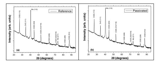
Fig. 4. (a) and (b) shows the XRD diffractograms of reference and passivated solar cells, respectively. The relative intensity peaks of CIGS related peaks for both the reference and the passivated solar cells remains unchanged.
