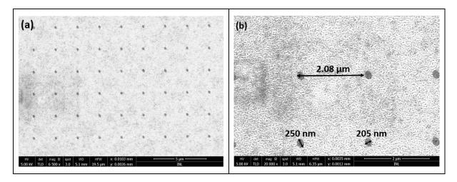
Fig. 2. SEM images of nano-contacts on the  $Al_2O_3$  rear passivation layer: ; (a) shows the well-ordered pattern of the nano-contacts; (b) shows the pitch, the consecutive distance between two nano-contacts and the approximate longer and shorter dimensions of the elliptic nano-contacts are shown
