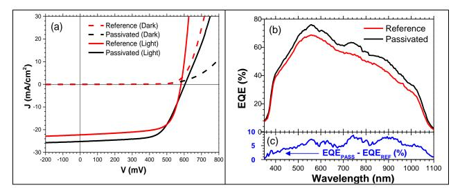
Fig. 6. (a) J-V and (b) external quantum efficiency (EQE) plots for reference and  $Al_2O_3$  rear passivated CIGS solar cells. (c) Absolute difference of EQE (in %) between passivated and reference solar cells. CIGS absorber layer thickness for both types of cells is approximately 500 nm.
