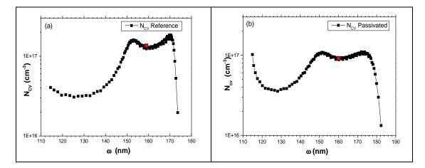
Fig. 7. Variation of the charge carrier concentration along the width of the depletion region for the (a) reference and (b) passivated solar cells. The red spots in the graphs shows the values for  $\omega$  and N extracted at 0 V bias voltage.
