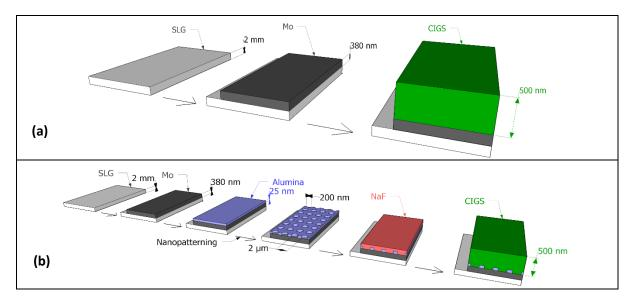
Fig. 1. Sequence of deposition steps (upto CIGS deposition) for (a) Reference and (b) Passivated Cells
