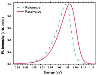
Fig. 8. Photoluminescence measured at 6 K under an excitation power of  $\sim$  3 mW for the reference and Al<sub>2</sub>O<sub>3</sub> rear passivated samples.
